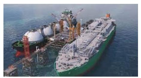
The project to develop and operate an LNG receiving facility off the coast of Gujarat, India, is being managed by Swan Energy. The Jafrabad FSRU is India's first newbuild Floating, Storage, and Regasification Unit (FSRU).
